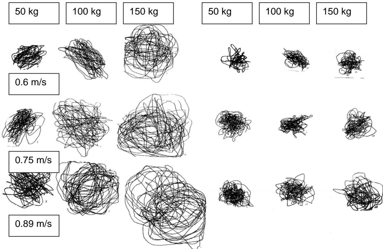
**Figure 3 Recordings of codend movements as a function of speed (horizontal) and catch size (vertical).
