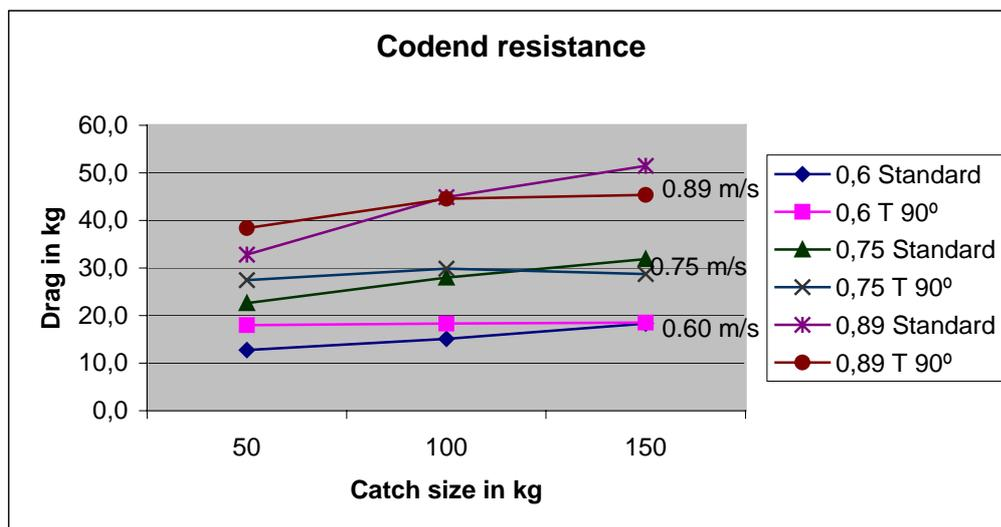
Diagram 2 The relation between catch size and drag in two different codends (no. 2 and 6) at 3 different towing speeds.
