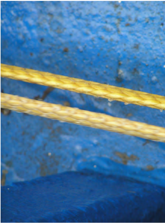
Illustration 7: Dyneema warps, new one upper and after one years of use
