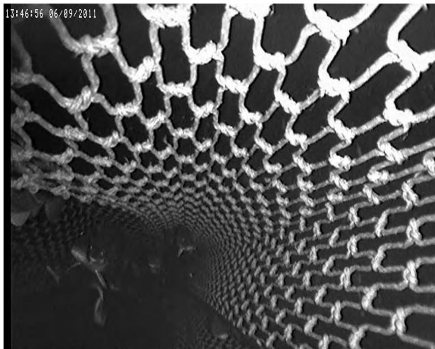
Illustration 6: Cod in the rear part of the belly of the Baltic cod trawl, note the open T90 meshes
