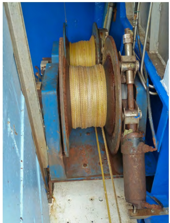
Illustration 8: Warp drums, note there are no warp guides
